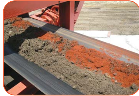
ViroSoil™ Technology installation and ViroBind™ application to dredge spoils.
