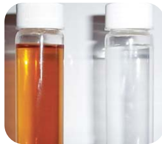
ARD at the Aqua Forte site before and after treatment with ViroMine™ Technology reagents.
