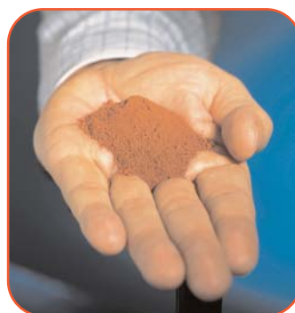
ViroChrome™ reagent was applied in powder form (it may be also applied as a slurry or in pellet form depending on the application).
