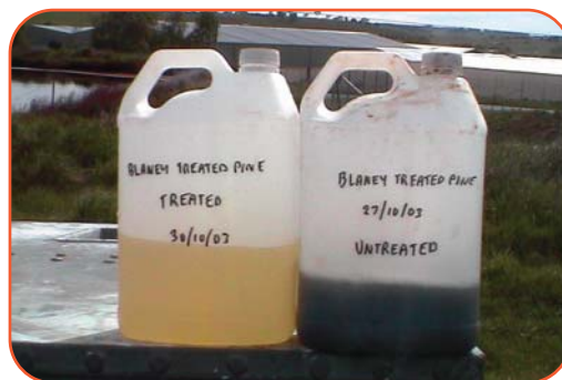
Figure 7 – Visual improvement in water quality before treatment (right) after treatment with ViroBond™ reagent (left).
