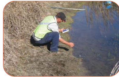
Water testing of the leachate pond prior to implementing ViroFlow™ Technology
