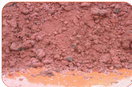
Figure 3 - Treated CCA stockpile after ViroFlow™ Technology Treatment application (wet weather during treatment produced some pooling)
