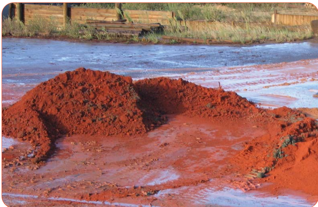
Figure 4 - Treated CCA stockpile after ViroFlow™ Technology Treatment waiting to be disposed of to landfill
