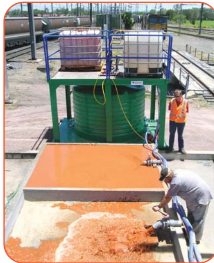
The inert sludge produced from ViroFlow™ Technology treatment.
