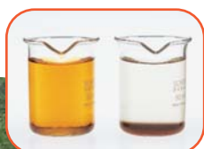
Water contaminated by AMD – before and after ViroMine™ Technology treatment
