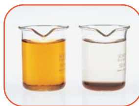
Water contaminated by AMD before and after ViroMine™ Technology treatment.
