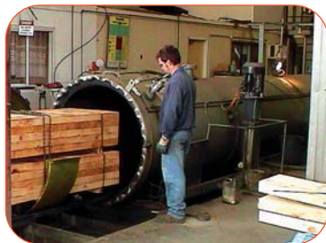
Left: Timber being treated with copper chrome arsenate. Right: Leachate from stored timber is contaminated with heavy metals.
