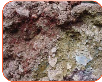
Photos showing sulphidic, acid generating rock and in-situ soil remediation in progress.
