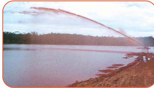
The ViroMine™ reagent was applied by a simple direct addition method as in the example shown above.
