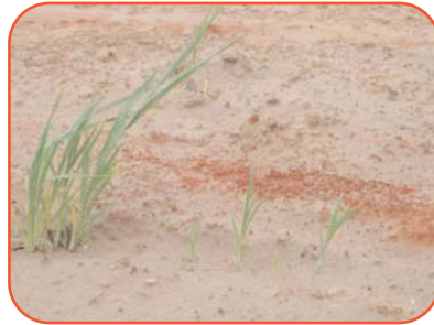
Figure 2. The germination of grass in the acid tailings after mixing the Acid B™ residues, remaining after water treatment, into the exposed tailings beach.
