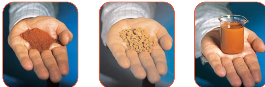
Virotec's reagents can be applied in powder, pellet or slurry form.
