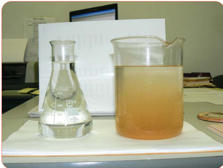
Figure 3: Treated process water (left) and raw process water (right).
