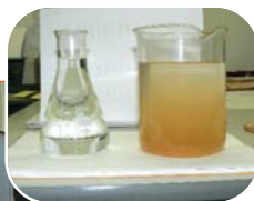
Treated process water on left and raw process water on right (above) View of installed water treatment system (left)
