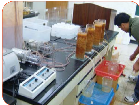
Figure 4: Filter columns being tested at Geoenvirontec's laboratory.
