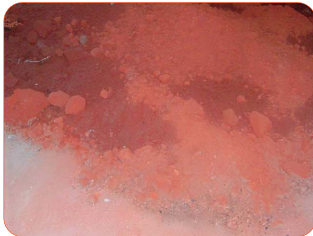
Electroplating waste treated with ElectroBind™ reagent and ready to be disposed to landfill.
