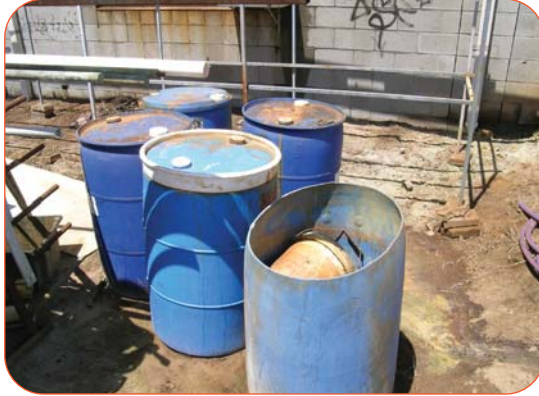
Electroplating waste leaking from containment drums into the soil from which it could be transported to nearby ecosystems during future rainfall events.
