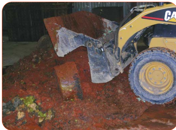
ElectroBind™ reagent was mixed with the solid electroplating waste with a Bobcat.
