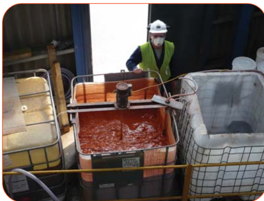
Figure 5: Close up of ElectroBind™ and mixer prior to dosing.
