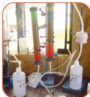
Conducting ViroFilter™ Passive Treatment trials at Gilt Edge Mine. The cells that gave the results overleaf were much larger – these small cells were subsequently used to help understand the limits of the method.
