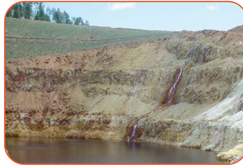
One of the contaminated pit lakes – with flowing ARD visible to the right.
