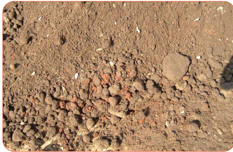
Figure 2 - ViroBlend™ reagent mixed with the waste product
