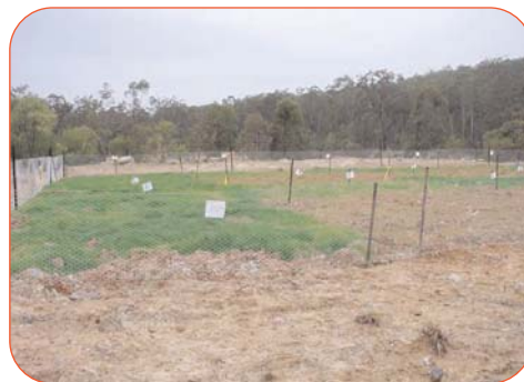
Figure 10: This photo shows the effect of revegetating waste rock with native grasses after treatment with ViroMine™ Technology (centre) in relation to untreated contaminated waste rock (foreground)
