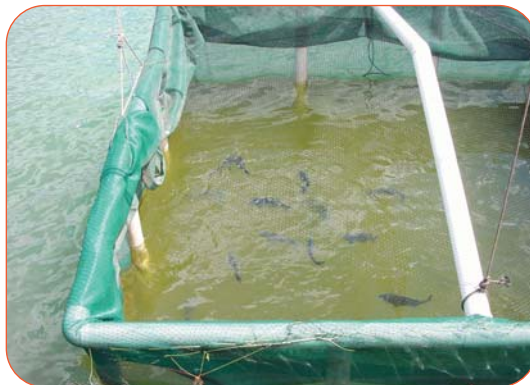
Figure 7: The silver perch in this photo are being used as toxicity indicators in mine water treated with ViroMine™ Technology
