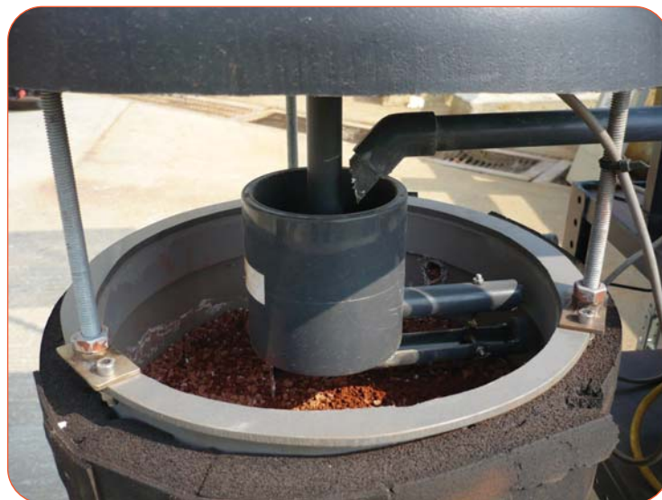
Figure 5: Close-up view of the ViroFlow™ Technology filter with acid- and iron-adjusted wastewater dispersed over the head of 2-6mm porous ElectroBind™ pellets.
